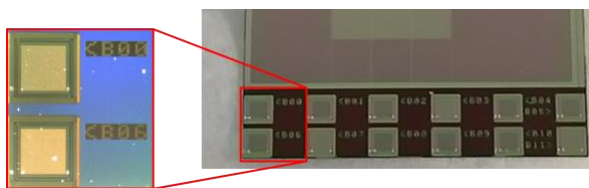
Figure 6. Photo of the test structures on the SiPDA wafer.
